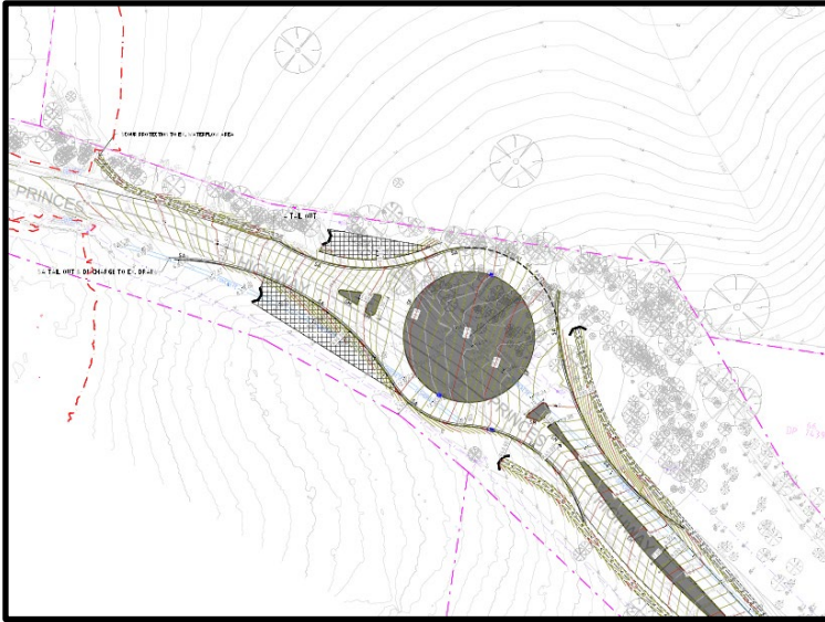
Figure 2: Section of the detailed design of the proposed roundabout configuration
